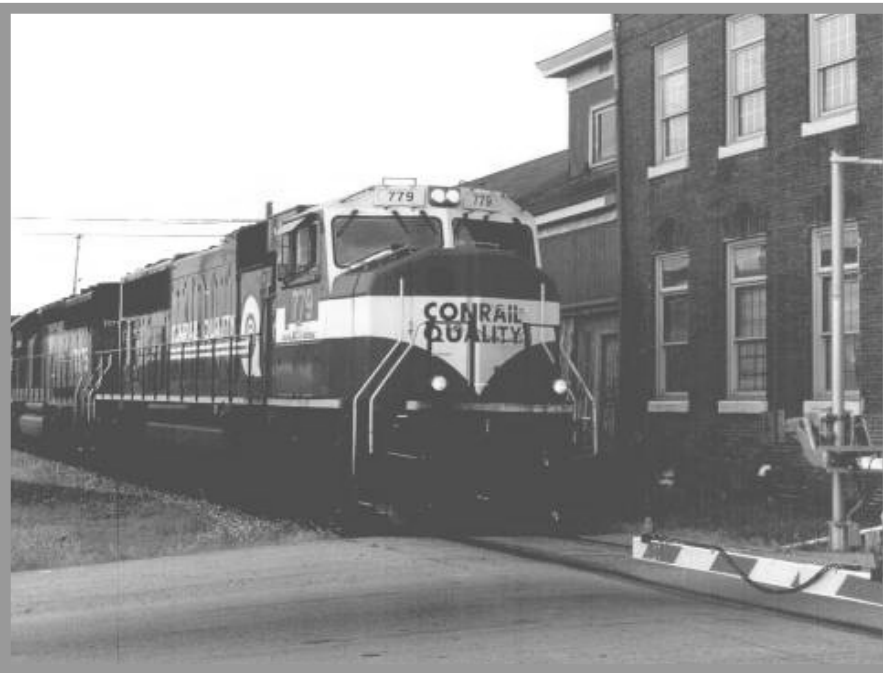
The second train by the L&N depot in Hopkinsville during the May Chapter meeting was southbound CSX Q597. The lead unit is CSX's ex Conrail SD70MAC still sporting CR's blue and white paint. The old L&N freight station is in the background. May 19, 2003 color print by Wallace
